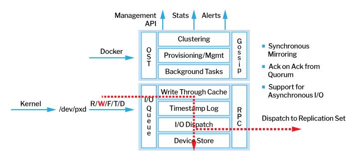
When a PX-Enterprise volume is exposed at the host, it appears as a local block device. This means that as long as the host is alive, the volume is attached to that node.
