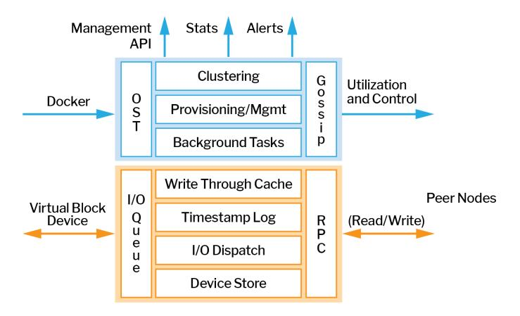
Each container gets a separate block device and separate queues that enable container granular data services and fine-grained quality of service.
